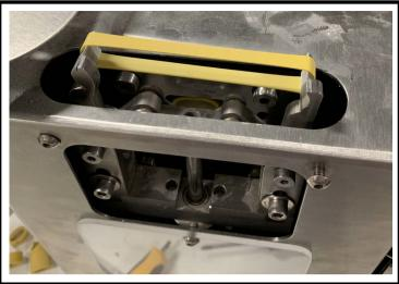
9 Finish by turning the safety shield and fastening the (2) socket head screws back into place. You are now ready to start auto loading of bands.
