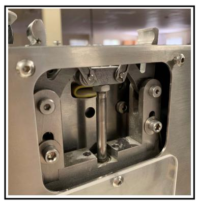
Turn the switch on the control panel to "AUTO" and then press the button labeled "CYCLE START" or trigger the sensor until a band is loaded onto the fingers.
