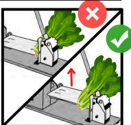
Adjust the height of the Receptacle Plate by removing the Plate Adjustment Pin. Once you've obtained the correct height, put the Plate Adjustment Pin back into place.
