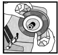
For normal use, feed ProTape® over Tape Rollers 1,2,3,and 4 (in that order).
